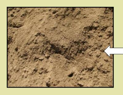
This is the mud we decided to use for construction. We got it from a few kilometers away from the school. By carrying out several tests, we found out that the clay content is around 35% and the sand was well graded. Good for us!
